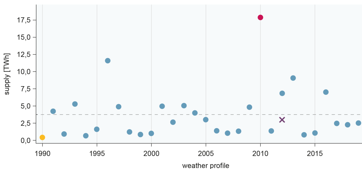
Figure 19: Heat production by methane-powered back-up boilers for weather profile years from the 1990-2019 period, in the National Leadership scenario in 2050. The yellow dot marks the year with the lowest number of hours, the red dot marks the year with the highest number, and the purple cross indicates the base scenario. The grey dotted line shows the 30-year average.
